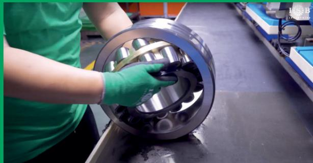
In these pages some images of the spherical roller bearings and the assembly phase. Beside some applications images.
