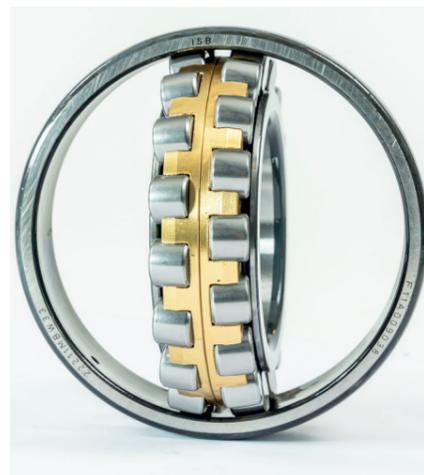
bore spherical roller bearings. Standard spherical roller bearings are neither sealed nor greased, and can be lubricated with oil or grease. Most radial spherical roller bearings have a circumferential groove and three holes in the outer ring for lubrication, the presence of which is identified by the suffix W33. Spherical roller bearings are suitable for use at operating temperatures up to +120 °C.
